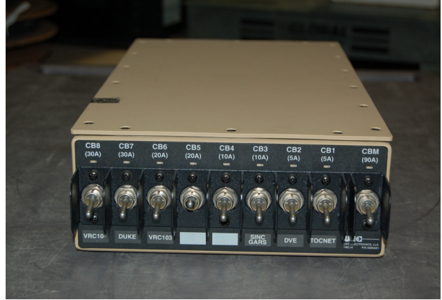
Vehicle Power Distribution Unit (PDU)
